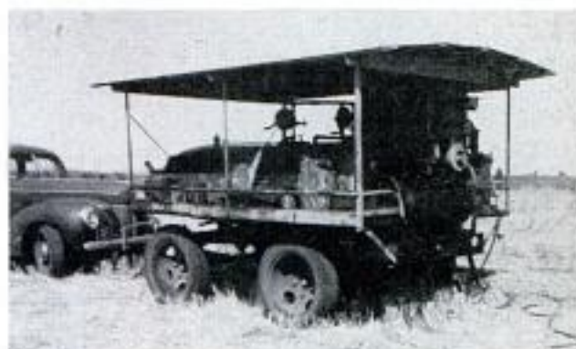
Another farmer rigged up this trailer, complete with sunshade. Loaded on the trailer are modern facilities for fueling and greasing all farm machinery
